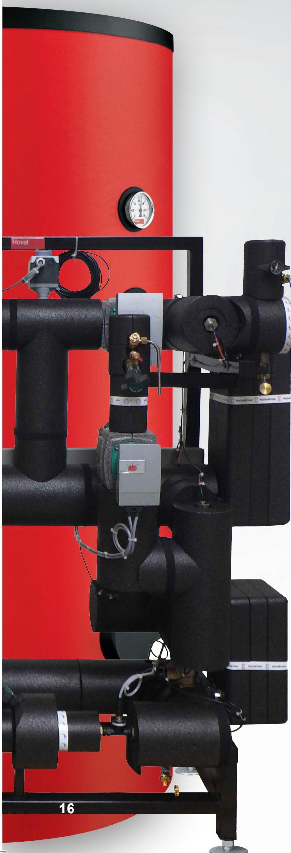
Domestic water heating in the continuous flow principle with 2 heat exchangers. Reduction in lime precipitation by controlling the heating charging temperature via a 3-way valve.
